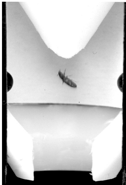
Fig. 2. An insect drops through a cutaway EGPIC sensor head. The insect snapped its own picture in mid-fall when it intersected the infrared beam (between the dark semicircular transducers), triggering an electronic flash.
