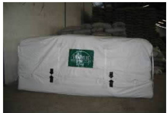
Fig. 6 Bio-generated atmospheres for the control of cocoa beans insects utilizing respiration of cocoa beans in a hermetically sealed cocoon.
