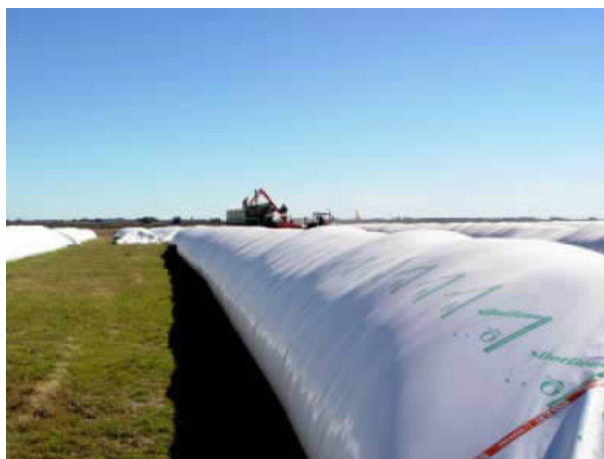
Fig. 1 Picture of a 200 – tonne capacity (60 m long and 2.74 m diameter) hermetic storage plastic bag (silo-bag).
