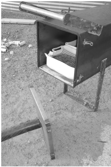
Fig. 12 Internal view showing AIP trays with plastic mesh
