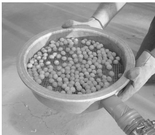
Fig. 4 Deep phosphine chamber – tablets loaded onto mesh tray.
