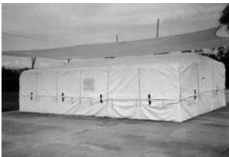
Fig. 3 Moisture migration has been solved by placing a reflective cover over the cocoons.
