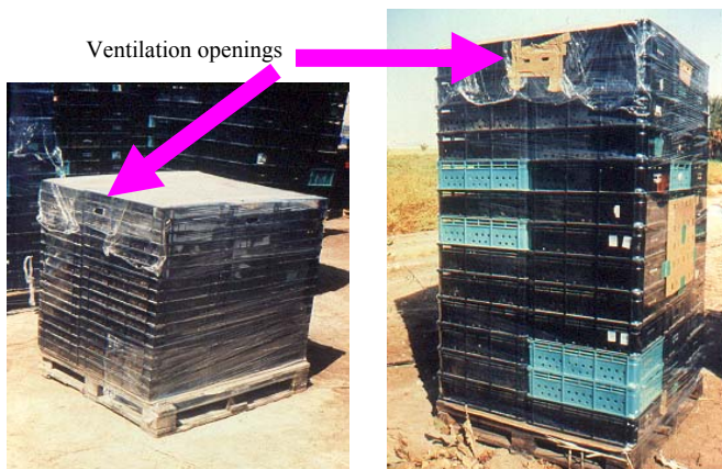
Figure 2. Two types of shrink film covered pallets for ripening Medjool dates using solar energy. Note the small ventilation opening to prevent condensation on trays located at the top layer.
